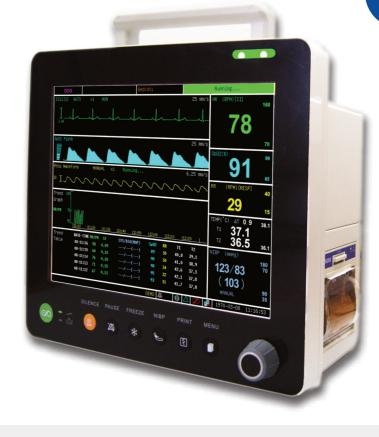
The PM6000V is a cost-effective, multi-parameter patient monitor, providing a reliable measurement on patient's SpO2, pulse rate, non-invasive blood pressure, temperature, 5-lead/3-lead electrocardiography (ECG) and respiration rate. Integ-rated sidestream technology ensures that the monitor can be used with intubated and non-intubated patients. 12.1 inch large display assures easy viewing of waveforms, numeric values and on-screen trending data for demanding veterinary facilities.
