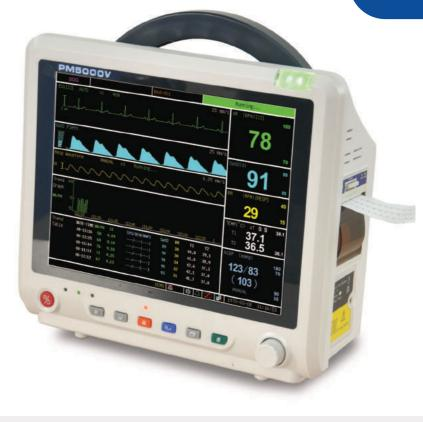
The PM5000V is intended to be used in veterinary clinics and hospitals to measurement patient's SpO2, Pulse rate, Non-invasive blood pressure, Temperature, 5-lead/3-lead electrocardiography (ECG) and Respiration rate. Optional parameters include two invasive blood pressure and capnograph (CO2). An internal printer is also provided as option.
