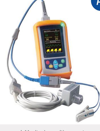
The UT100VC Vet Capnograph Monitor is a multi-parameter monitor that measures and displays capnography data and fractional inspired CO2 (FiCO2) values of intubated and non-intubated animals as well as respiratory rate, oxygen saturation (SpO2) and pulse rate. It combines semi-quantitative end-tidal carbon dioxide detection with veterinary pulse oximetry into one portable, durable and economical handheld monitor.
